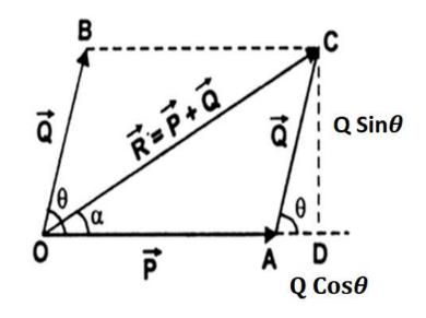
$$\tan \alpha = \frac{\text{CD}}{\text{OD}} = \frac{\text{CD}}{\text{OA} + \text{AD}} = \frac{Q \sin \theta}{P + Q \cos \theta}$$
